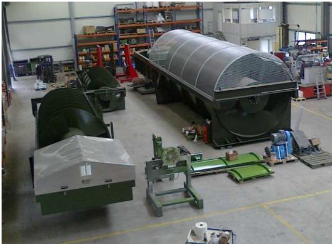
Figure 12: Screw turbines of various sizes in the factory, with and without covers
